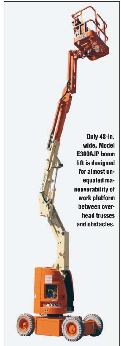
Only 48-in. wide, Model E300AJP boom lift is designed for almost unequaled maneuverability of work platform between overhead trusses and obstacles.
