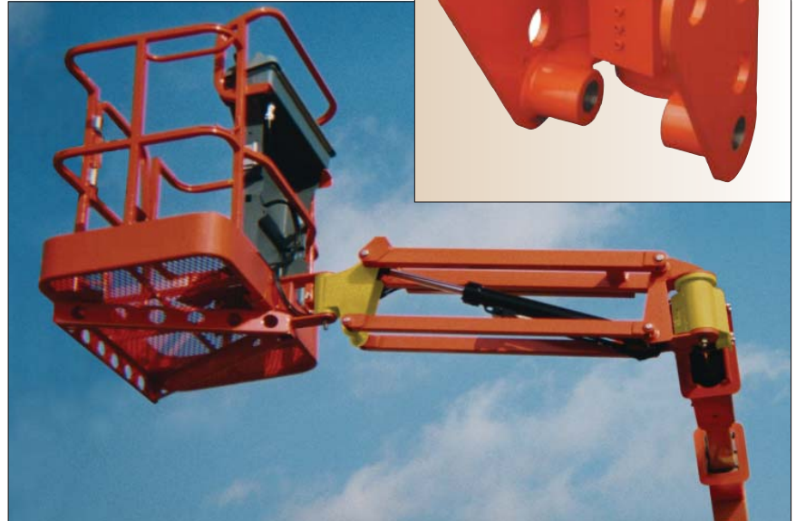
Rotary actuators between main and jib booms (at right) and between jib boom and platform (left center) provide extra boom articulation capabilities to move platform precisely over, under, and around obstacles. Inset shows rear view of L20-15 rotary actuator and mounting clevis used on boom lift, with actuator's large-diameter, drilled-and-tapped shaft flange at top right.
