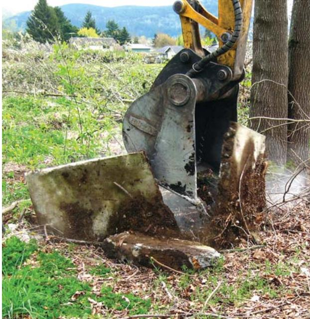
jaw and back of bucket that's designed with Helac's sliding-spline operating technology, which converts linear piston motion into powerful shaft rotation. The end caps, seals and bearings work in unison to keep debris and contaminants out of the inner workings of the actuator,
